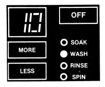
A number in the display shows the time in minutes remaining in that portion of the cycle indicated by the four sequence lights—Soak, Wash, Rinse, Spin. The illustration shown at the left would indicate 10 minutes of wash time.
